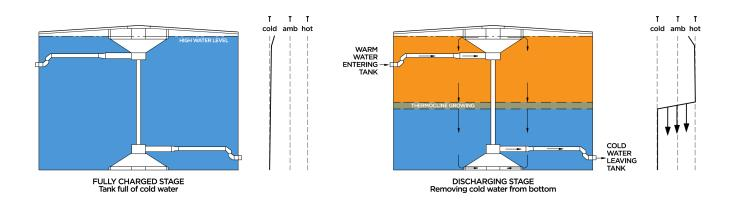
2. During off -peak periods, when electrical rates are low, the chilled TES tank is recharged. Warm water is withdrawn from the top of the Chilled TES tank, cooled with conventional water chilling units, and returned to the bottom of the tank.
