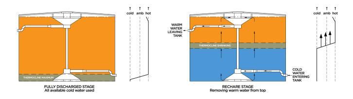
3. Hot Water TES tanks operate similarly. Properly designed diffusers distribute the flow within the tank to minimize mixing. The water naturally stratifies, with the lighter, warmer water floating on top of the colder, denser water.
