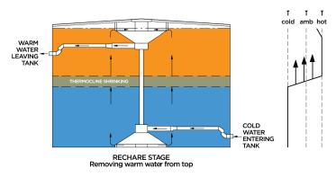
3. Hot Water TES tanks operate similarly. Properly designed diffusers distribute the flow within the tank to minimize mixing. The water naturally stratifies, with the lighter, warmer water floating on
