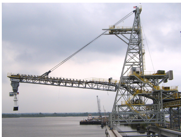
Figure 3. Ship loader moves alongside the vessel for distributed loading, minimising time at dock and demurrage costs.
